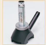
5. Using the scale factor (number of \mu\text{m} or mils per graticule division), calculate the coating thickness for each layer.
