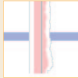
3. Using the P.I.G. make a cut, at right angles to the marker line, all the way down to the substrate
